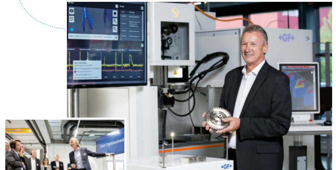
Pascal Boillat , Head of GF Machining Solutions, presents a Fir Tree Disk for an aerospace turbine at the Capital Market Day. This part is manufactured even more precisely thanks to the new EDM technology Spark Track.
