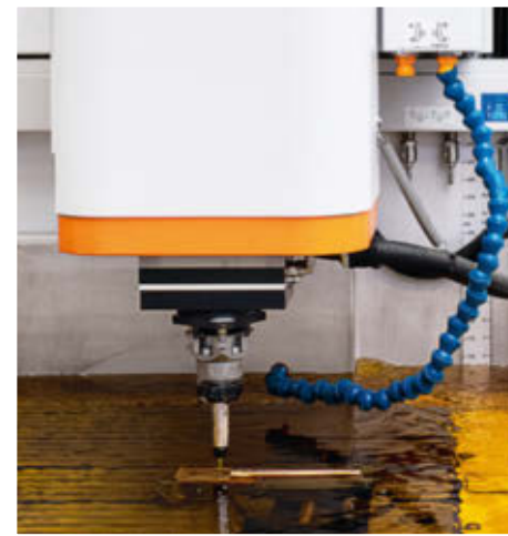
Since March 2021, CERN has relied on the CUT P 800 to produce small components for the LHC particle accelerator. The enormous amount of energy contained inside the machine allows for more precise metal processing than a milling machine.
