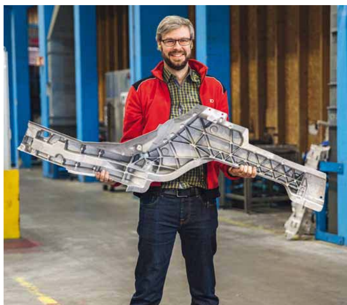
Marc Hummel with the 1.43 meter sill frame member
