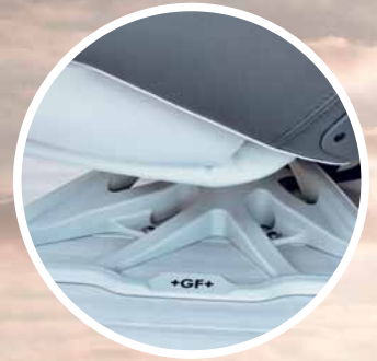
An agile electric speedster for town and country: the “Oasis” has large glass panels and clad front wheels. GF Automotive supplied a bionic aluminum seat support for this car.
