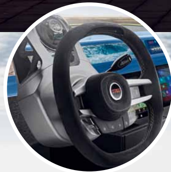
The “XchangE” is a fully electrically powered luxury tourer. The futuristic steering wheel – complete with lightweight support made by GF Automotive – can be electrically stowed in the middle of the vehicle.
