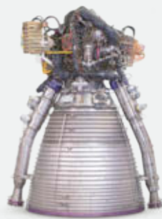
The Vulcain 2.1 engine is 3.7 meters high and weighs over 2 metric tons.
