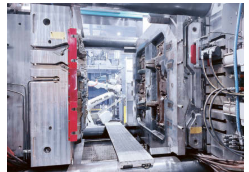
↑ This die-casting machine, located at the GF plant in Altenmarkt (Austria), is also capable of being used in big casting.
