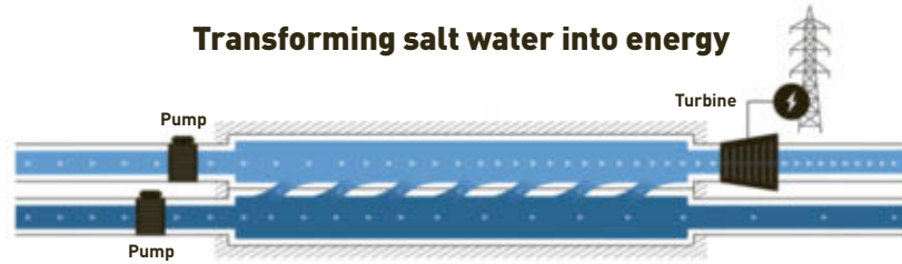
How the SaltPower concept works: a system pumps fresh water and salt water through two tanks separated by a membrane with pores so tiny that only water can pass through them. Seeking a natural balance, the fresh water automatically moves through the membrane and mixes with the salt water to equalize the salinity levels. This controlled water transfer creates a build-up of pressure that powers a turbine and generates electricity.
